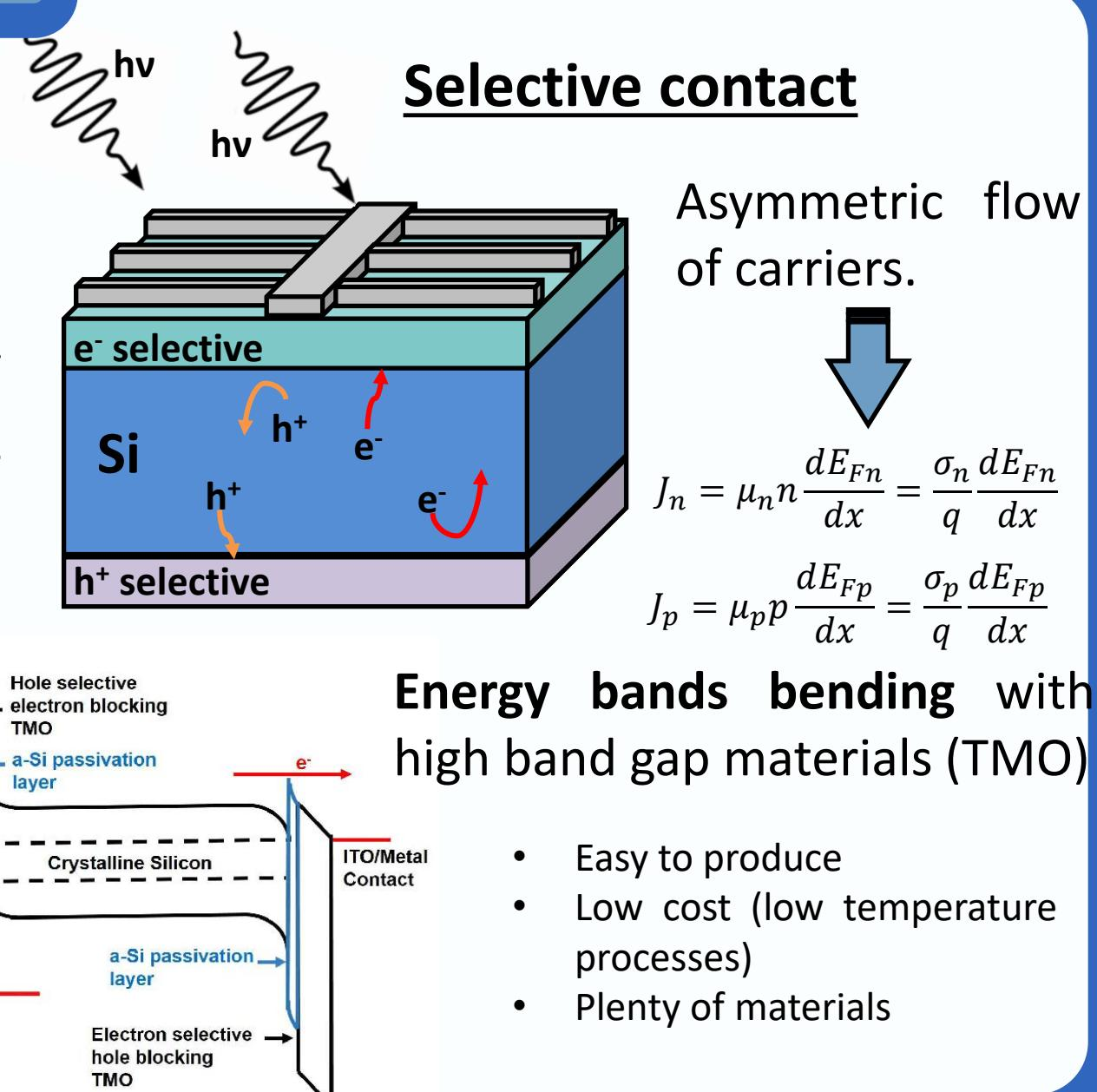
Energy bands bending with high band gap materials (TMO)
