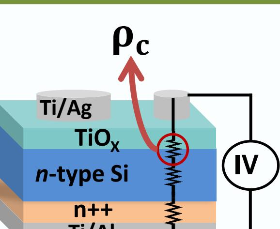
Cox&Strack samples to measure the  $\rho_c$  of  $\text{TiO}_x/\text{n-Si}$  junction. Three different sputtering time (6min, 4min and 2min), each one grown at 150 °C or 200 °C.
