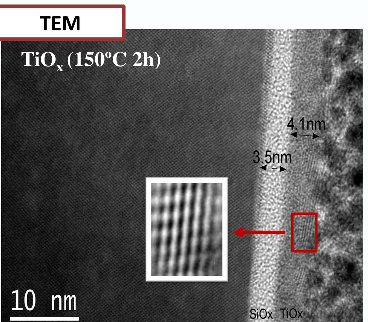
TEM image shows an amorphous  $\text{TiO}_x$  with some regions that portray embedded nanocrystal. Furthermore, a thin  $\text{SiO}_x$  film has regrown, probably due to the diffusion of  $\text{O}_x$  inside the Ti film.
