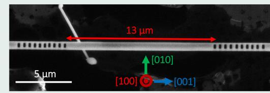
SEM images of the  $\beta\text{-Ga}_2\text{O}_3\text{:Cr}$  nanowire on a TEM grid, showing the optical cavity and DBRs.
