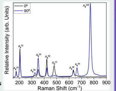
Raman Spectra allows us to know the crystal orientation and relate it with the anisotropic refractive index for NW by angle-dependent Raman analysis.
