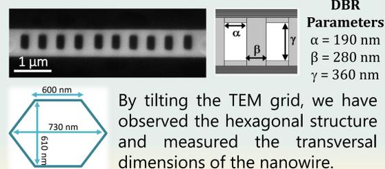
By tilting the TEM grid, we have observed the hexagonal structure and measured the transversal dimensions of the nanowire.
