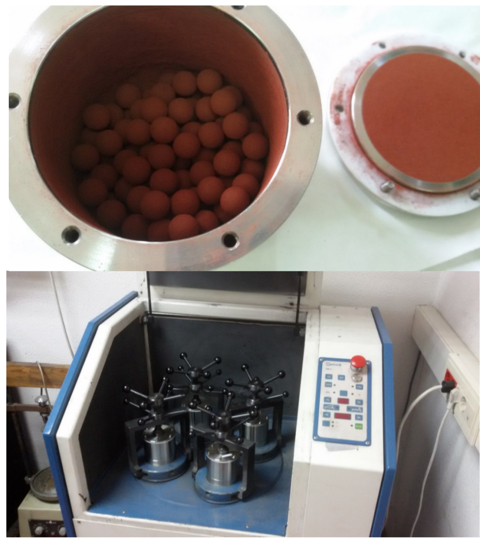
Hematite and zincite powder are high energy ball milled
