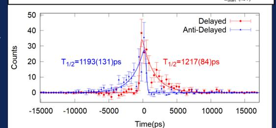
Figure 7. (Top) gamma-gamma coincidence matrix recorded in the  $\text{LaBr}_3$  detectors. (Bottom) TAC distribution for the 174-348 gamma-gamma coincidence. Lifetime is obtained from the fit of the slope.
