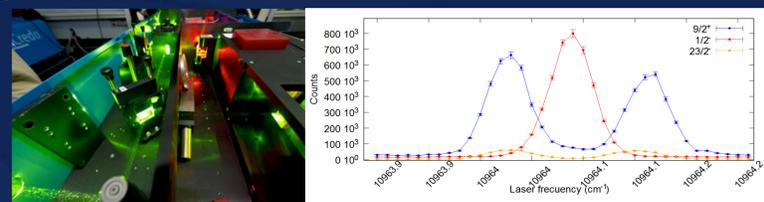
Figure 3. (Left) RILIS setup. (Right) Scan of  $^{129}\text{In}$  isomer production, monitored by  $\gamma$ -rays in our experimental setup.
