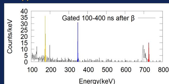
Figure 6. Gamma-ray spectrum recorded in HPGe detectors in a delayed coincidence with the beta-detector.
