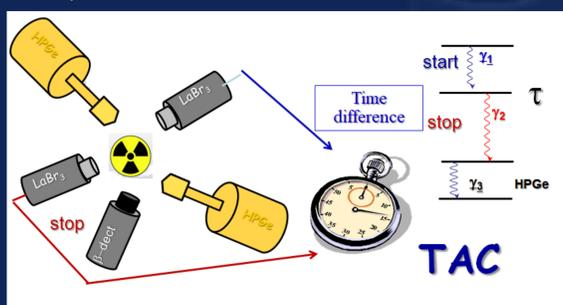
Figure 4. Schematic setup for the fast-timing technique. Timing information by the fast-scintillator detectors because of their fast time response. Commonly HPGe are include to gain selectivity thanks to their excellent energy resolution.
