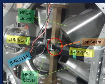
Figure 2. ISOLDE Decay Station(IDS). Detector setup used during the experiment IS610.
