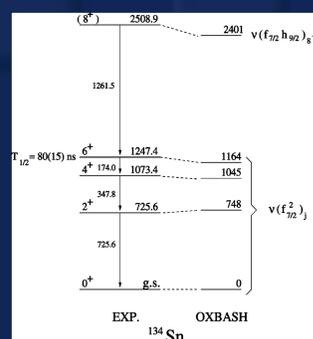
Figure 5. Level scheme of  $^{134}\text{Sn}$  observed in  $^{248}\text{Cm}$  spontaneous fission.[2]
