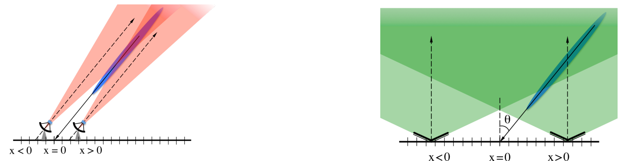
Fig. 4: Geometry of both Cherenkov techniques, IACTs (left) and WACDs (right), observing an air shower.
