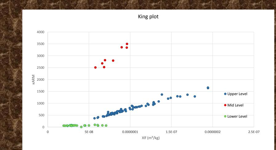
Since that we have samples where the dominant magnetic mineral is magnetite, the King Plot provides a means of assessing grain sizes. In this case, we have a typical distribution for small grains  $(0.1\mu m)$ .
