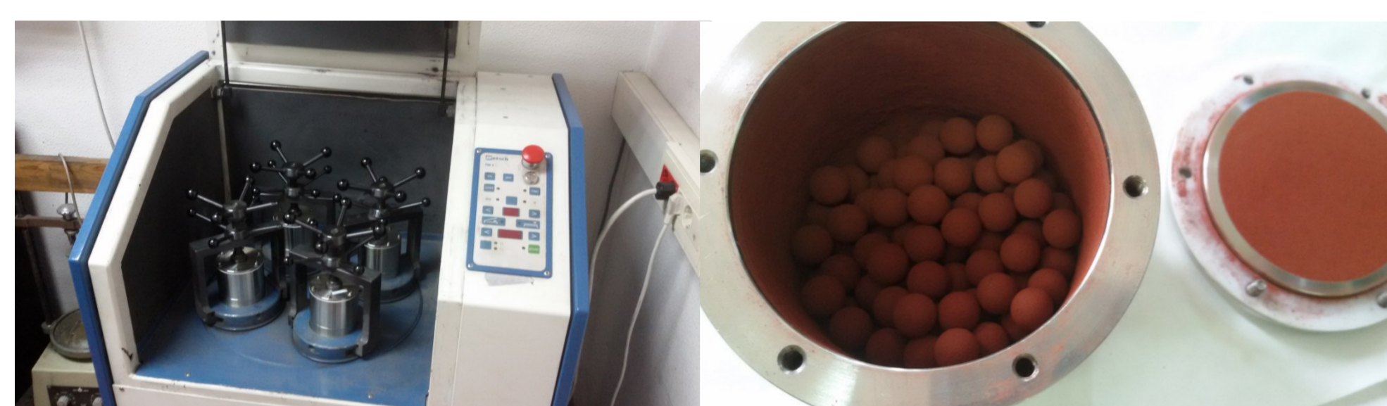
High energy ball milling hematite and zincite powder
