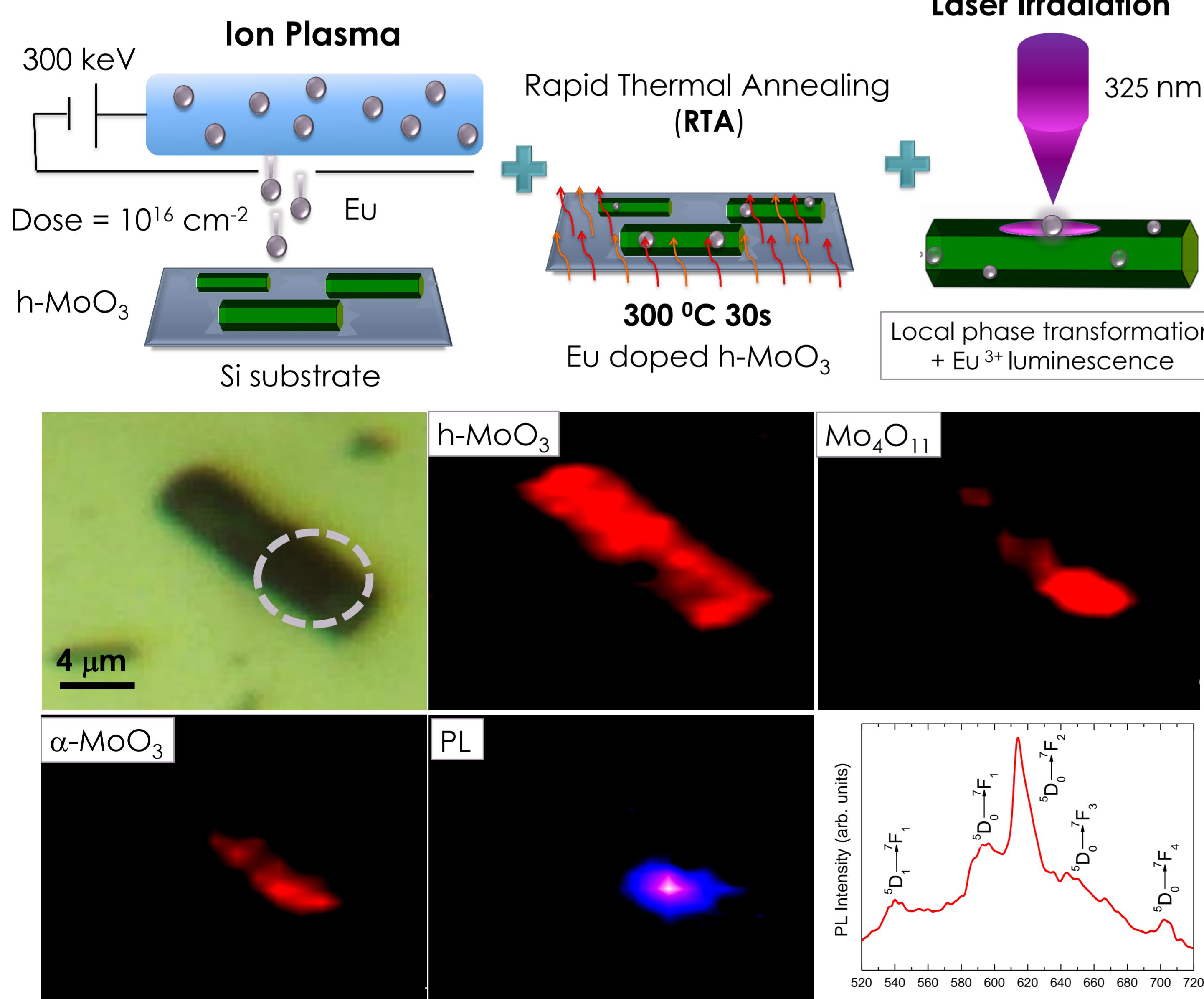
**Optical activation** of Eu ions implanted in h-MoO<sub>3</sub> can be effectively achieved by **laser irradiation**. Raman and PL mappings reveal that **Eu<sup>3+</sup> luminescence** emission is triggered by a h-MoO<sub>3</sub> to α-MoO<sub>3</sub> and Mo<sub>4</sub>O<sub>11</sub> phase transformation (P. Almodóvar et al. Appl. Phys. Lett. 113 (2018) 031902; CrystEngComm 20 (2018) 4954).
