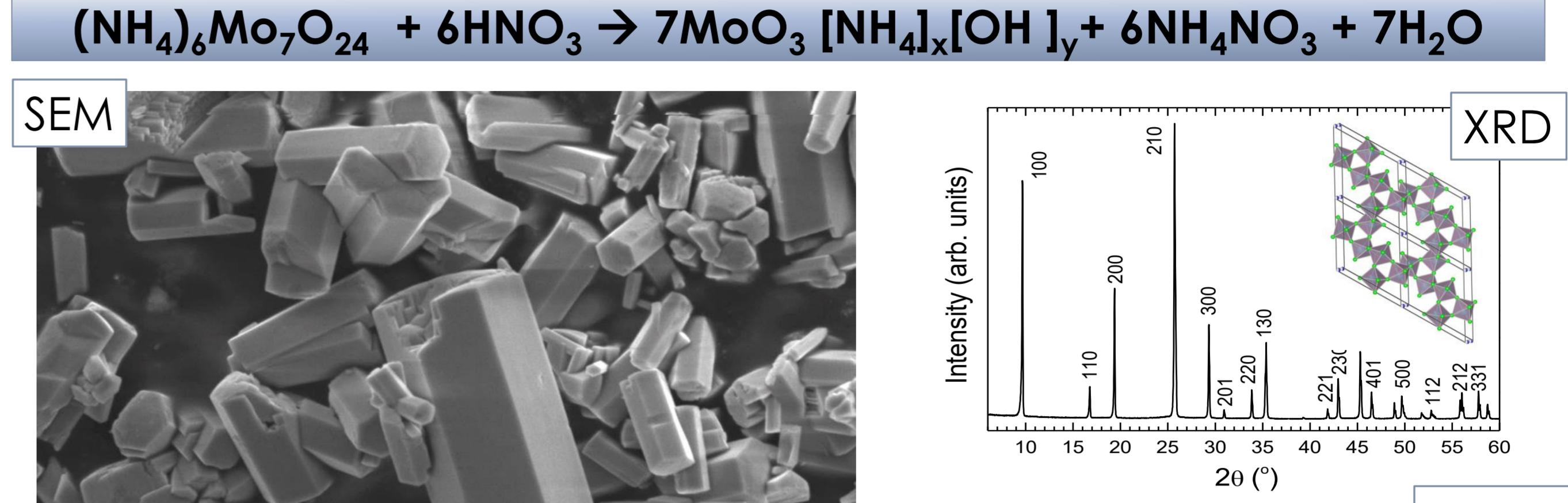
**Single crystal**, h-MoO<sub>3</sub> rods were obtained. Average size is ~1 μm x 5 μm, but can be adjusted modifying the synthesis conditions.
