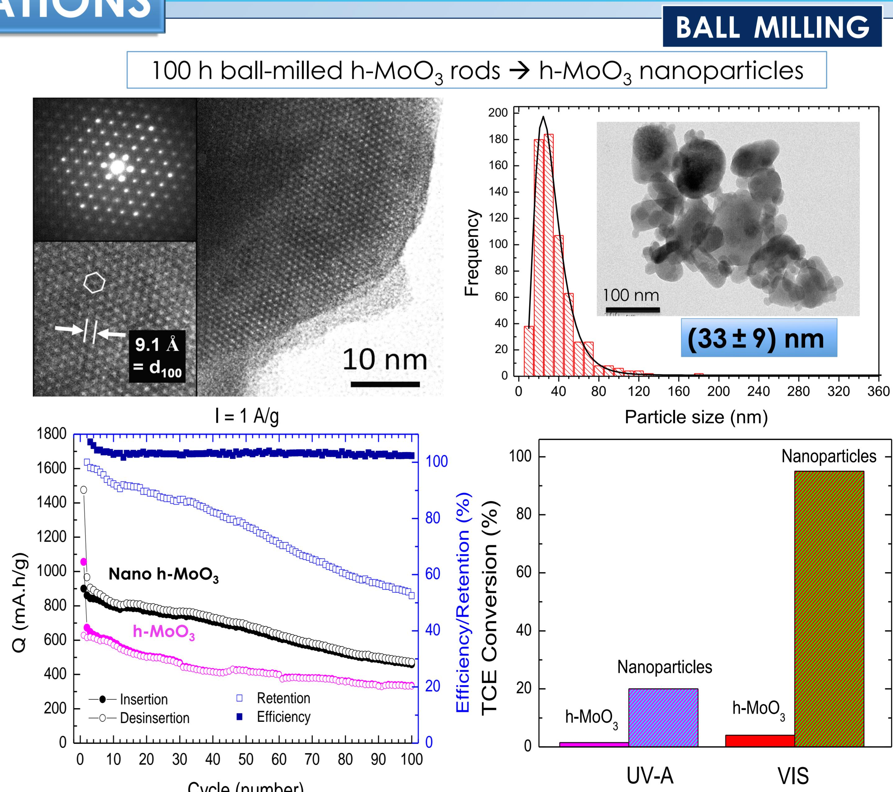
Increased **anode stability** as well as significantly improved **photocatalytic activity**, as compared to as-grown h-MoO<sub>3</sub>.
