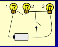
When switch is closed, bulb 2 will a. stay same brightness, b. get brighter c. get dimmer, d. go out.
